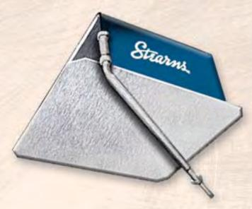
The Stearns magnet design produces a magnetic field that is not only deep enough for full penetration at the center of the conveyor, but also extends outward for complete tramp iron removal at the edges of the burden. Units are complete with a manually operated discharge arm for tramp iron removal. Also available in self-cleaning models.
